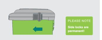
Depress red tab and slide both side catches completely forward.
