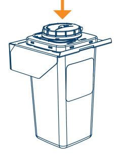
To lock the container in place, slide the tabs of the cover into the slots in the bracket.
